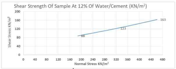
Figure 7: Shear Stress - Normal Stress (KN/m<sup>2</sup>) at 12% Water/Cement
