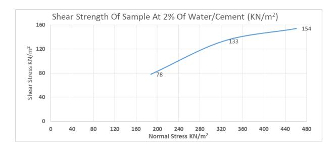
Figure 2: Shear Stress - Normal Stress (KN/m<sup>2</sup>) at 2% Water/Cement
