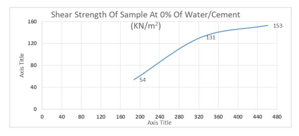
Figure 1: Shear Stress - Normal Stress (KN/m<sup>2</sup>) at 0% Water/Cement
