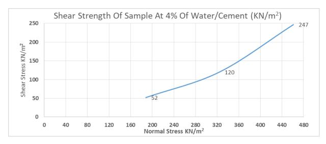
Figure 3: Shear Stress - Normal Stress (KN/m<sup>2</sup>) at 4% Water/Cement
