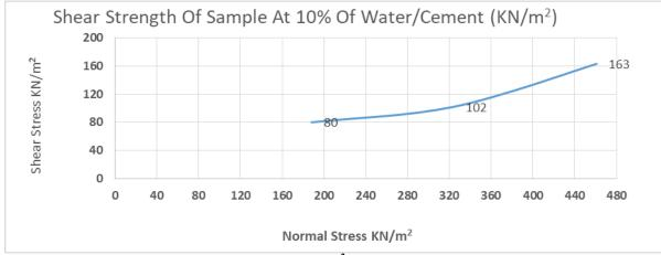
Fig. 6: Plot of Shear Stress against Normal Stress (KN/m<sup>2</sup>) at 10% Water/Cement
